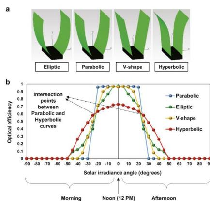
Fig. 2. (a) The concentrator models that were analysed with ray tracing software. (b) The optical efficiency of the concentrator models as a function of various irradiation angles. Reprinted from Momeni & Ni (2018).
